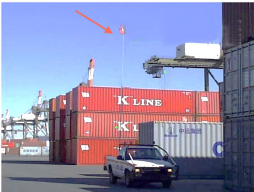
Figure 9. Elevated & Illuminated Poles for small vehicles, photo courtesy of ILA~USMX Joint Safety Committee
