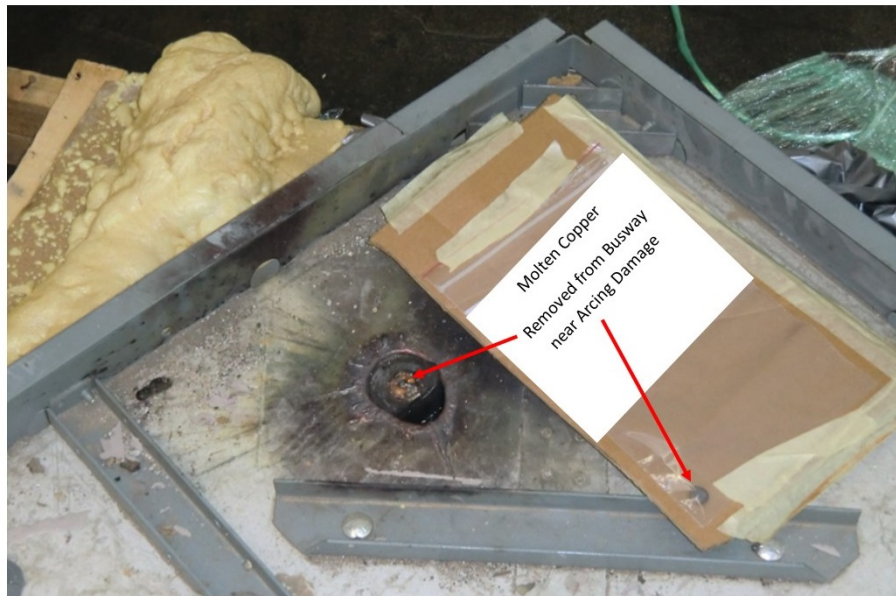
Penetration via impact drill into a 277 Volt AC Bus Duct
